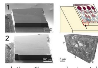
For structure data acquisition we used block-face scanning electron microscopy with the Zeiss Auriga® Crossbeam Workstation (FIB-FESEM) on Os / U- stained tissue embedded in epoxy resin. XY-resolutions of <10 nm/px with good membrane contrast, and a Z-resolution of 10 nm (milling rate) with virtually no image distortion makes perfectly aligned 3D structure data available in 10 nm isotropic re-
